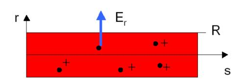
We assume cylinder symmetry and no variation in s-direction. In case of a homogeneous space charge distribution within the
