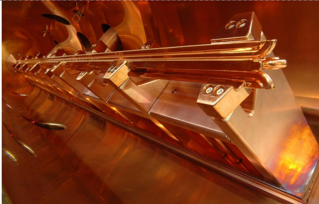
Deuterium - Uranium, length: 2.055 m, \beta_{in} = 0.0023 , \beta_{out} = 0.025 , res. frequency: 108.408 MHz 4-rod RFQ at SARAF/Israel
